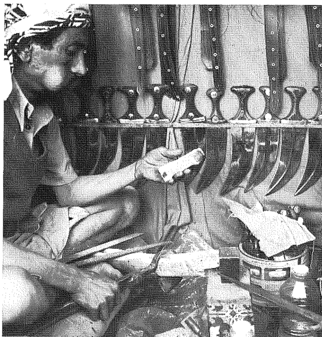
Dagger handle being carved from rhino horn in North Yemen
