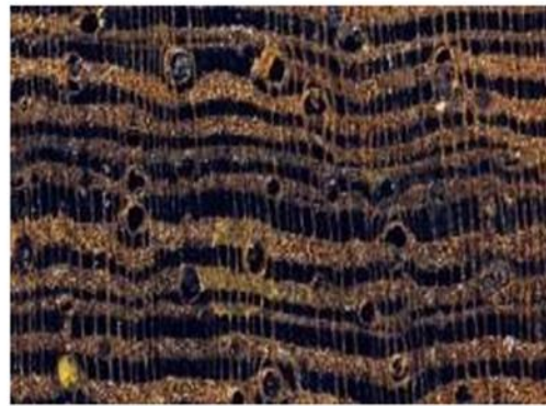
Parenchyma band larger than or the same with pore diameter
