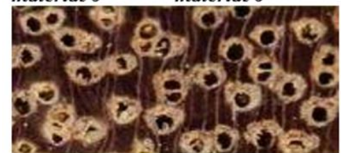
Solitary and multiple vessels in Ironwood ( E. fordii ). Source: Reference material 7
