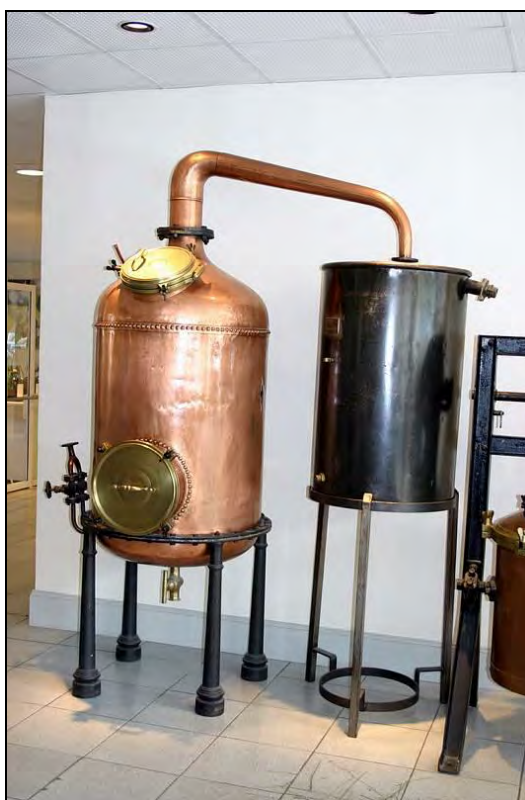
Figure 16. A simple distillation apparatus for extraction of volatile oils 17
