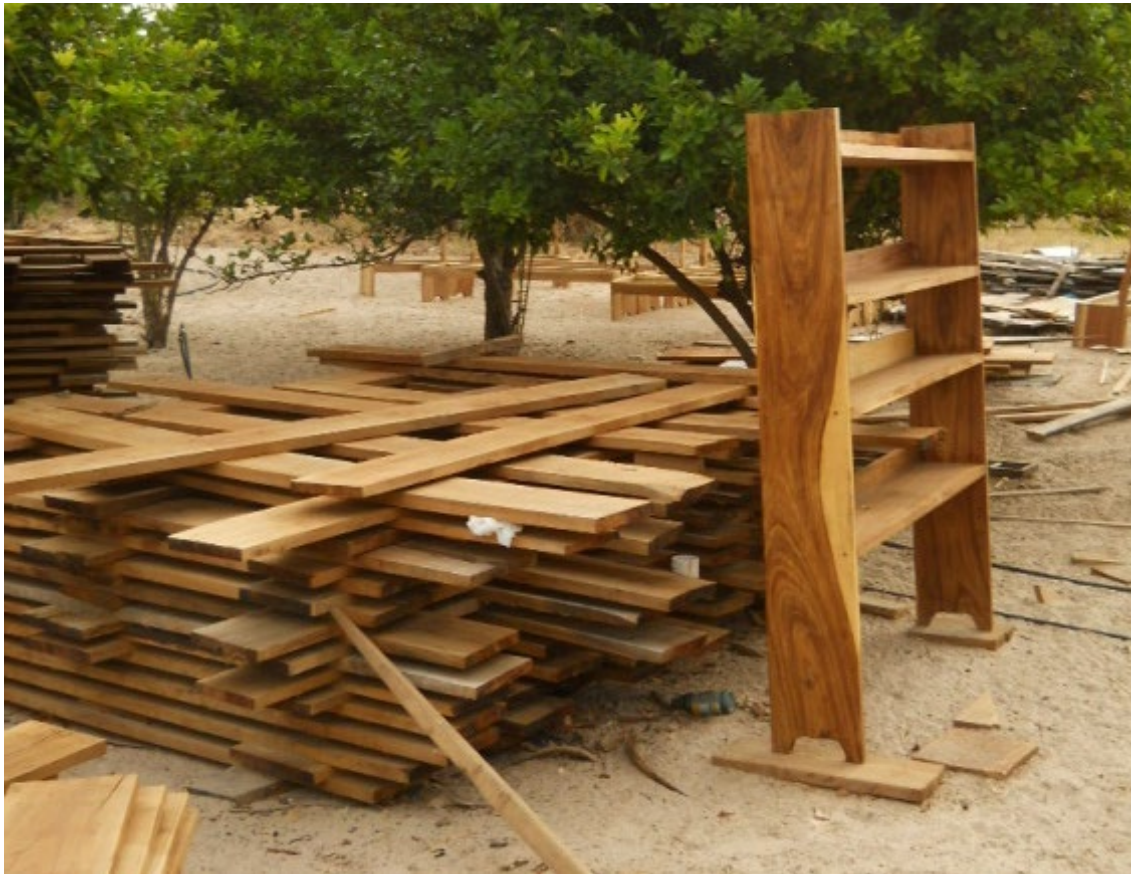
Figure 2: Kiaat P. angolensis planks showing the pale sapwood and the darker heartwood
