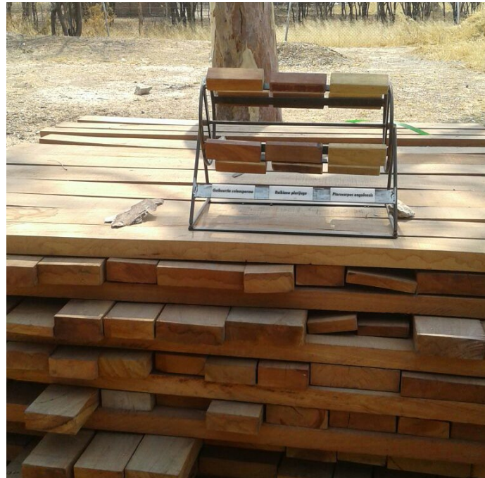
Figure 25: Timber wheel being used to identify the timber species during an inspection (Source: K. Nott)
