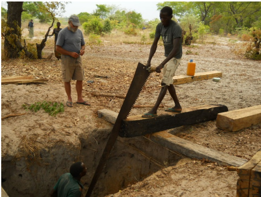
Figure 10: Pit sawing of Kiaat P. angolensis logs
