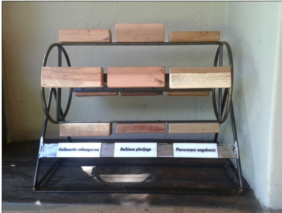
Figure 8: Timber wheel developed to assist with the identification of timber species during inspections
